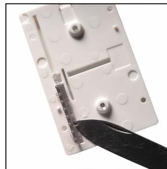
Snap out the light pipes with a flat tool
